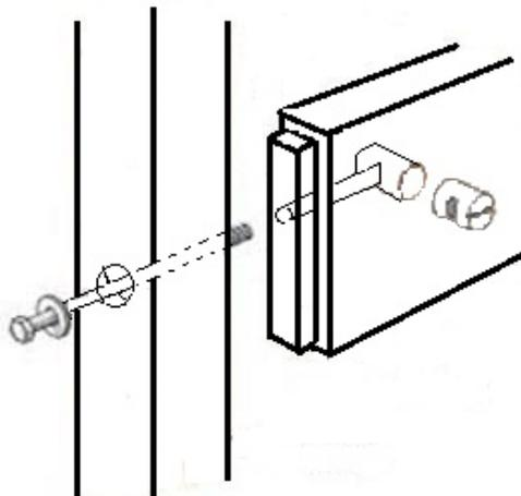
The barrel nut must be inline with the bolt. After insertion the bolt will thread through the nut to secure.
