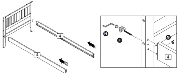
Step 6: Attach the footend using hardware parts F, G and H.
