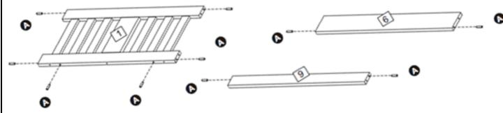
Step 3: Attach the right headend post (2) and left headend post (3) to the headend panel (1) and headend rail (9) using hardware parts E and H.
