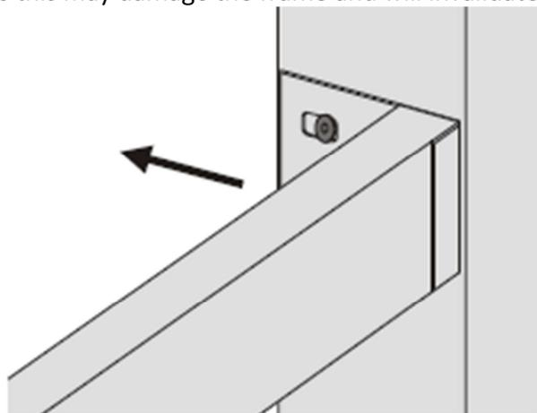
Step 5: Place hardware part D onto every end of each slat (7) then press firmly into the side supports (5). DO NOT use any power tools as this may damage the frame and will invalidate any claim.
