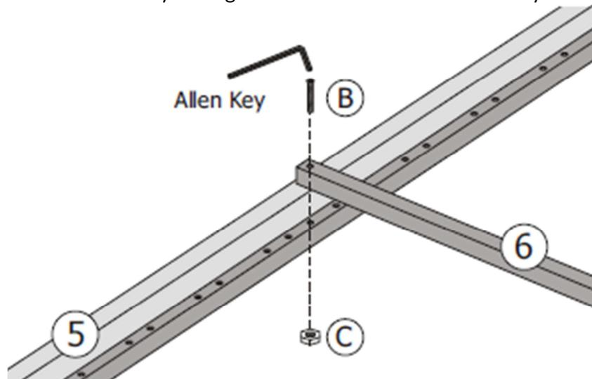
Step 4: Adjust both side supports (5) into the inner direction until the screws reach the end of the hole as shown. Tighten the screws for both side supports and the mid support. DO NOT use any power tools as this may damage the frame and will invalidate any claim.
