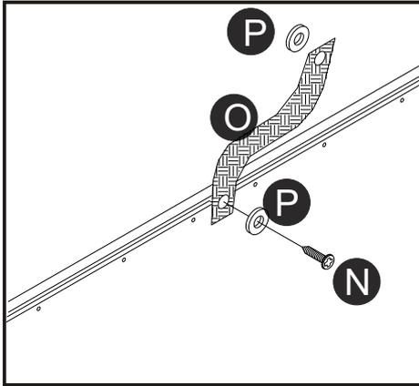
The product should be fixed to the wall using the wall strap.
