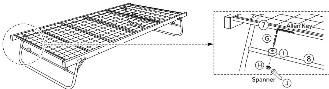
**STEP 7:** Hook the bar to the Trundle Leg (8) to lock it when in the open position.
