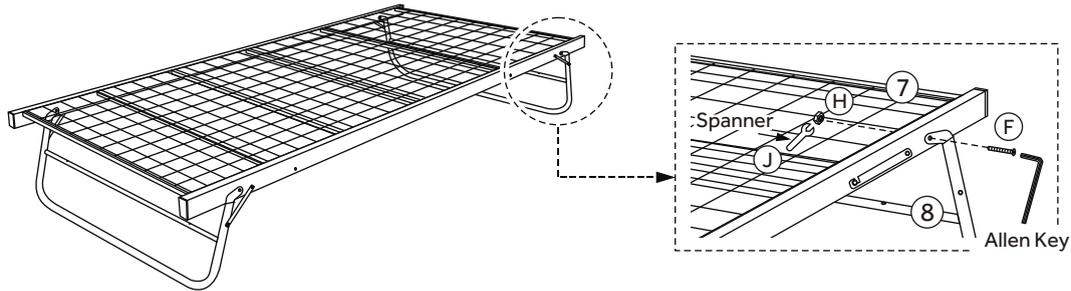
**STEP 6:** Fix hardware part (I) to the Trundle Legs (8) using hardware parts (G) and (H)
