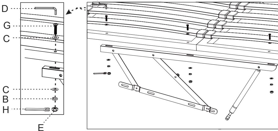
Use fixings (E), (C), (B) & (G)- tighten the bolt by using allen key (D) with spanner (H).
