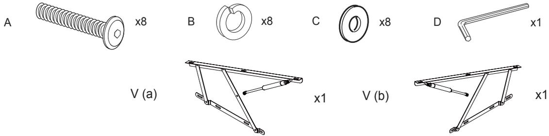
CHECK THIS DIAGRAM AND IF ACCESS IS NEEDED FROM RIGHT SIDE OF BED, FIT THE PAIR OF LIFT MECHANISMS TO **LEFT** SIDE OF THE BED. BOLT INTO THE HOLES MARKED (L) WITH RED LABELS. THE MECHANISMS ARE LABELED V (a) & V (b) - PLEASE CAREFULLY FOLLOW THE DIAGRAM BELOW.
