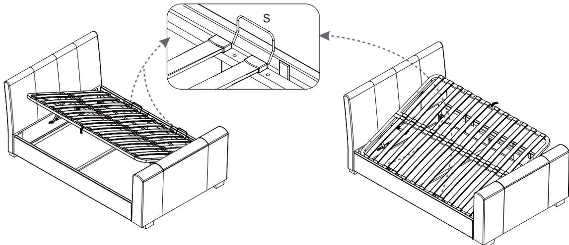
NOTE: Place mattress on slat-frame when frame is down. Lift with strap & close with strap which should always be accessible. Slowly lift frame by the lifting strap taking care to not lean over the bed because if the mattress is thin & light, frame will rise quickly. To close bed, push gently away from lifting strap side and down at the same time. The frame will close, speed of closing depends on weight of mattress so always keep fingers well clear of the metal frame.
