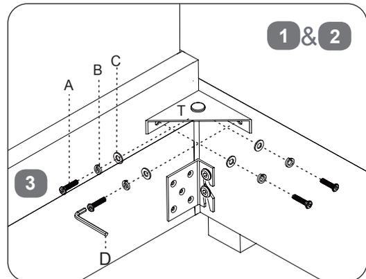
Fit the angle brackets (T) into the corners of the Headboard & Footboard (1&2) and Side Panels (3). Fit the bolts (A) with washers (B&C) through holes in angle brackets (T) as shown. Fit all four brackets but do not tighten bolts yet.
