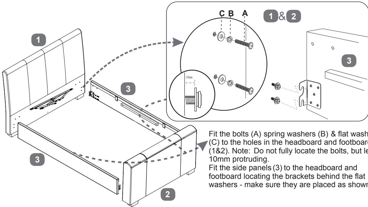
Fit the bolts (A) spring washers (B) & flat washers (C) to the holes in the headboard and footboard (1&2). Note: Do not fully locate the bolts, but leave 10mm protruding.
