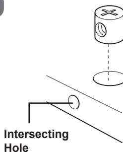
When they are supplied and are part of the assembly of this bed, ensure that barrel nuts are fitted the correct way so the hole is facing towards the intersecting hole.
