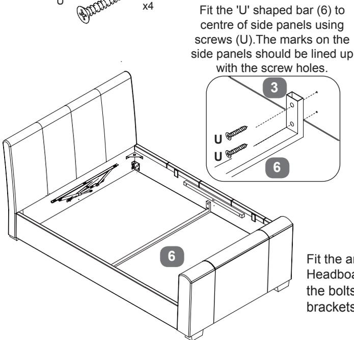
Fit the 'U' shaped bar (6) to centre of side panels (3) using screws (U). The marks on the side panels should be lined up with the screw holes.
