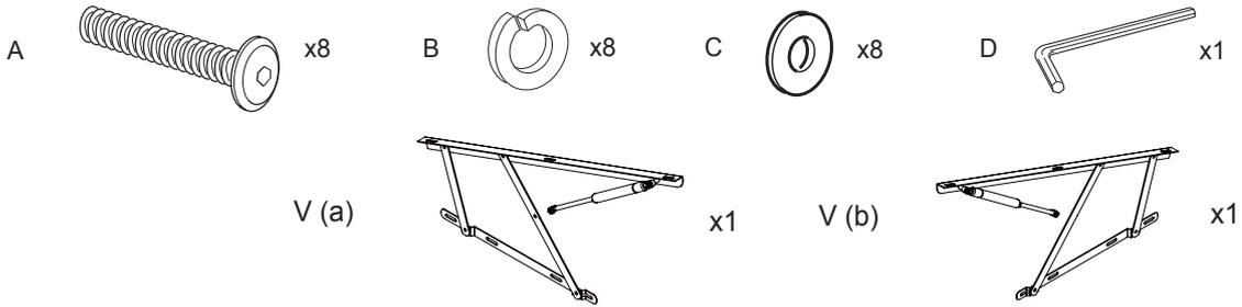
CHECK THIS DIAGRAM AND IF ACCESS IS NEEDED FROM LEFT SIDE OF BED, FIT THE PAIR OF LIFT MECHANISMS TO **RIGHT** SIDE OF THE BED.
