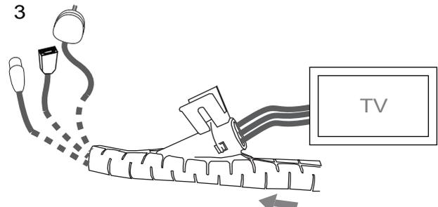
Feed tube in this direction—hold clip firmly in place
