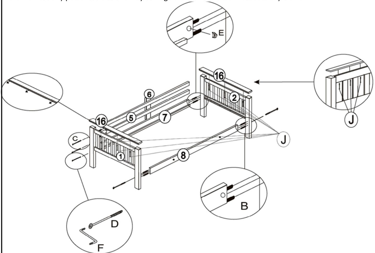
Step 3: Connect the bottom headend (3) and bottom footend (4) with the bottom back side rail (9) and bottom front side rail (10) using hardware parts B, D, E and F.
