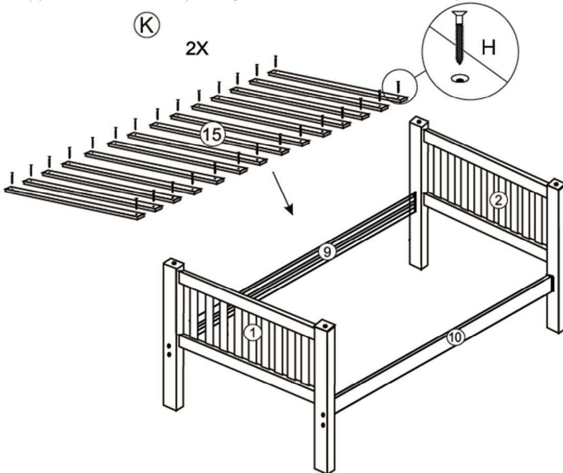
Step 5: Connect the two frames together using hardware parts A and H with a screwdriver (not provided).
