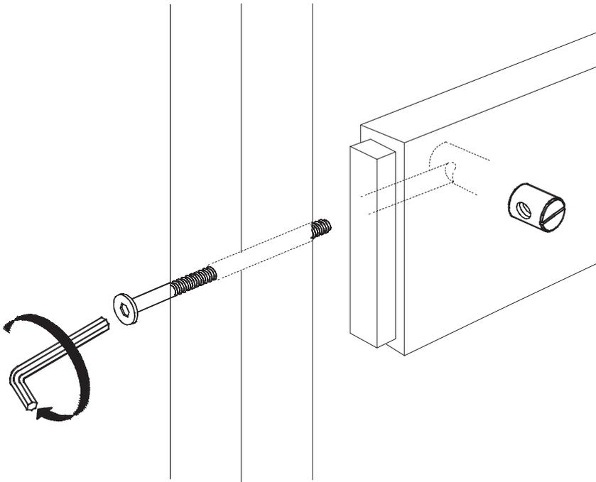
The barrel nut must be in line with the bolt. After insertion the bolt will thread through the nut to secure.
