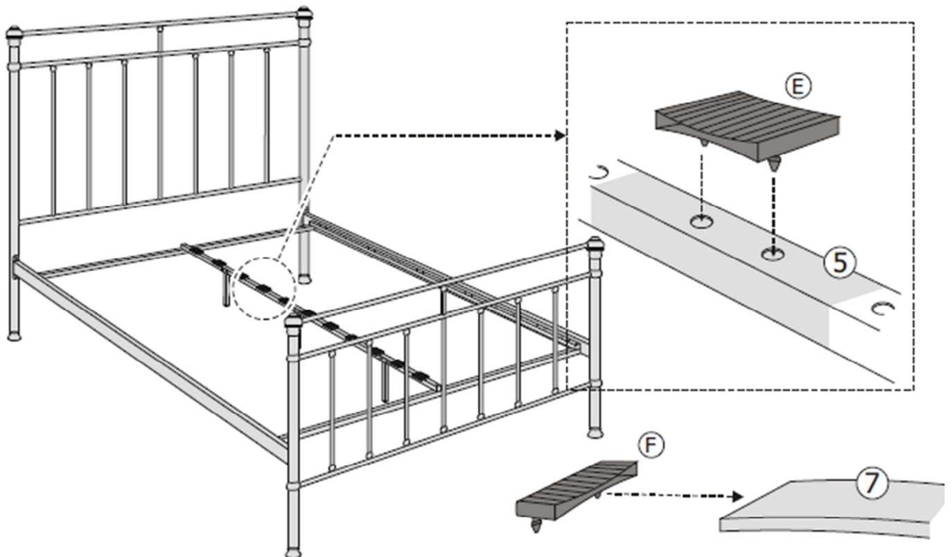
Step 6: Insert the slats (7) to hardware part E and press firmly into the side supports (3). Insert hardware part I.
