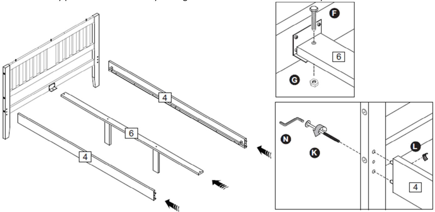
Step 7: Attach the footend using hardware parts K, L and N and fix the centre rail (6) in place using hardware parts F and G with an M11 spanner (not provided). DO NOT use any power tools as this may damage the frame and will invalidate any claim.
