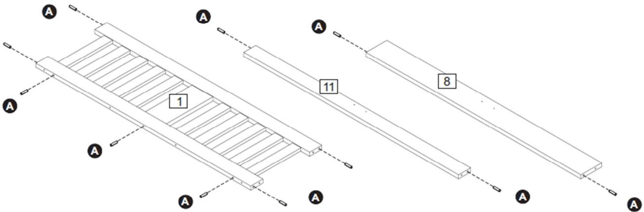
**Step 3:** Attach the right headend post (2) and left headend post (3) to the headend panel (1) and headend rail (11) using hardware parts J and N. DO NOT use any power tools as this may damage the frame and will invalidate any claim.
