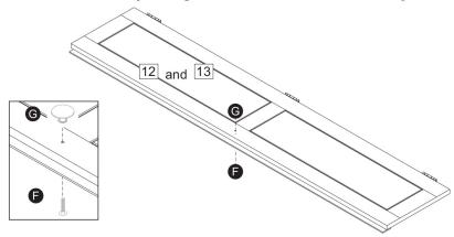
**Step 9:** Attach the right door (12) and left door (13) using hardware part B and a screwdriver (not provided). **DO NOT use any power tools as this may damage the frame and will invalidate any claim.**
