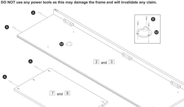
**Step 4:** Attach the front frames (6), base panel (7) and shelf panel (8) using hardware part D and a screwdriver (not provided).
